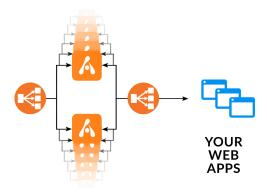
Virtual WAF works in auto-scaling groups to support bandwidth up to AWS limits
